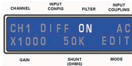
Figure 2.16 - 100kHz, Low-Pass Filter ON Display Setting
